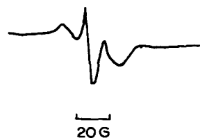
Fig. 3. The ESR signal of Tinuvin-622 after irradiation.
