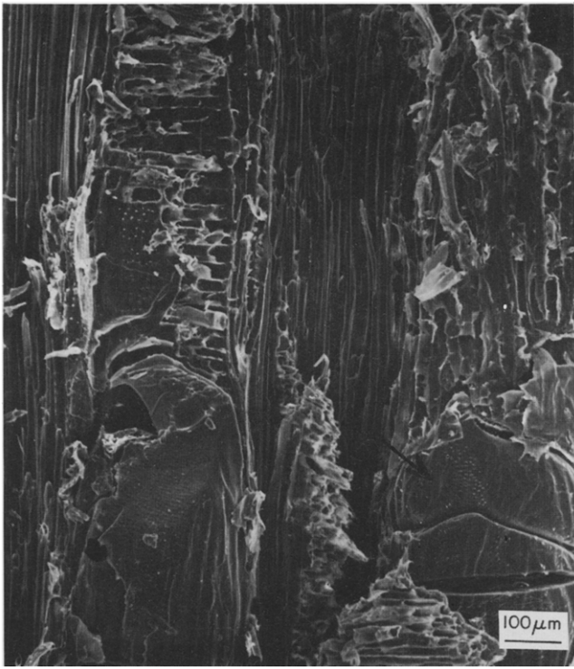
Fig. 11 Fractured surface on the wood–glue joint of Yellow Seraya bonded and tested by tensile shear under wet condition thirteen years ago. Adherend: 20 h boiled wood; arrow: a part of delaminated surface of glue cast
