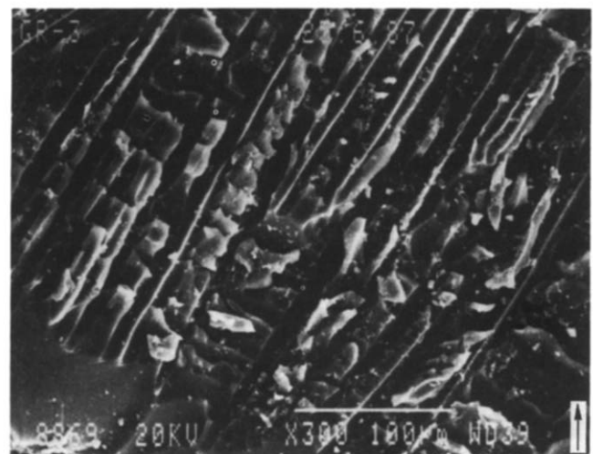
Fig. 6 Fracture surface of unexposed glass/epoxy specimen ( \times 300 ) Delamination is in arrow direction \uparrow
