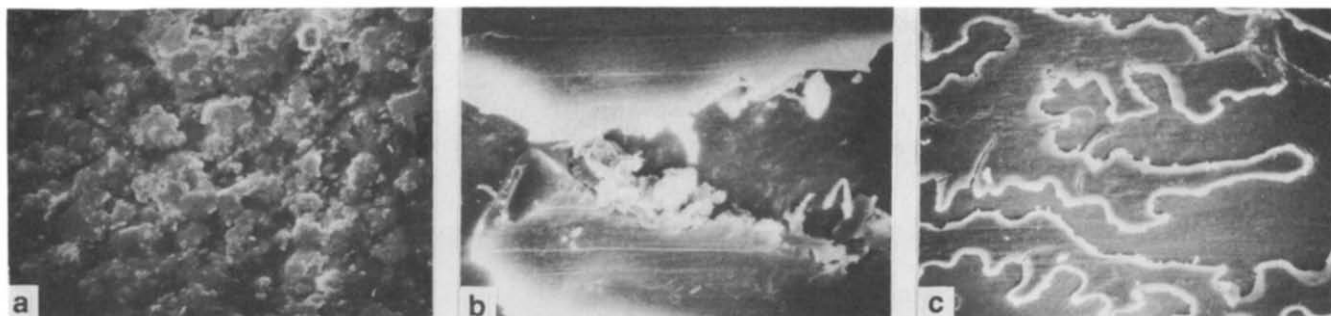
Fig. 6 Scanning electron micrographs of peel surfaces of Al joints bonded with: (a) 62:38 blend, \times 600 ; (b) 36:64 blend, \times 1200 ; (c) pure BMF, \times 150
