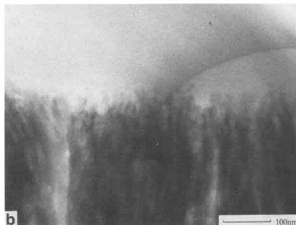
Fig. 5 (a) Cross-sectional TEM image of the interfacial region between adhesive/primer AF163-2K/EC3960 (at the top of the image), oxide (in the middle) and aluminium adherend for a high peel strength specimen ( 12.3 \text{ N mm}^{-1} ). (b) Cross-sectional high magnification TEM image of the interfacial region between adhesive/primer AF163-2K/EC3960 (at the top of the image) and oxide (at the bottom) for a specimen with high peel strength ( 12.3 \text{ N mm}^{-1} )
