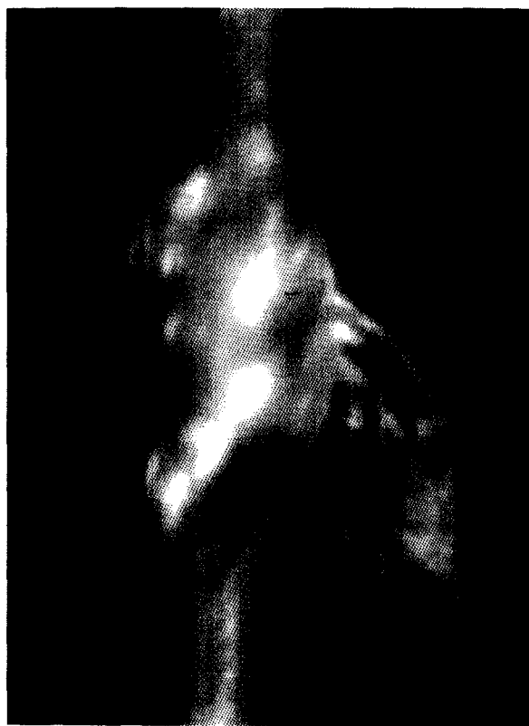
Figure 7 Matrix failure during the microbond test applied to an \text{NH}_3 -treated PTFE fibre/epoxy assembly
