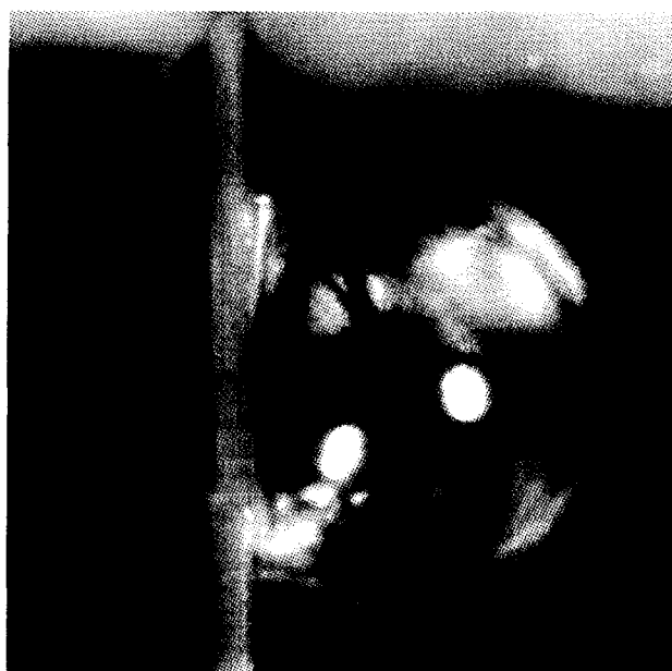
Figure 4 Non-axisymmetric resin droplet on an untreated PTFE monofilament
