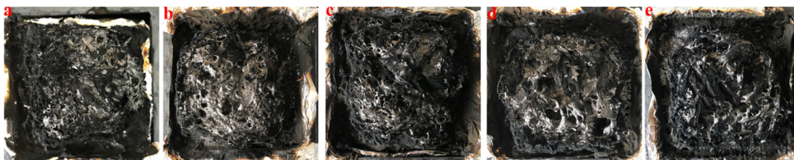
Fig. 8. Digital photographs of char residues (a. EP, b. EP5, c. EP10, d. EP15, and e. EP20).
