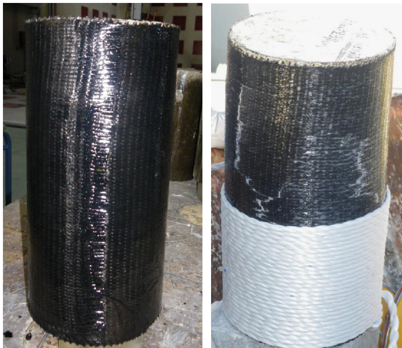
(a) Concrete cylinder after wrapping with GF-CNTRP (polymer S2WV_0.125%)
