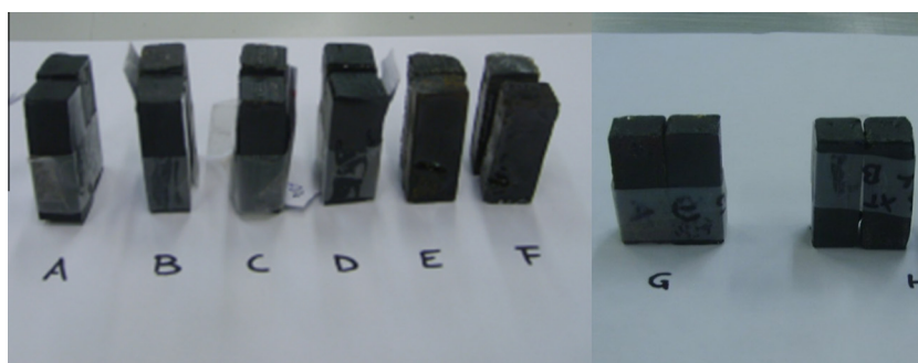
Fig. 8. Detail of failure of bonded joints occurred in butt joint tests.
