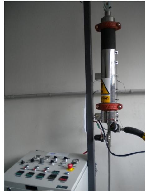
**Fig. 2.** Resin injection system – temperature and pressure control.
