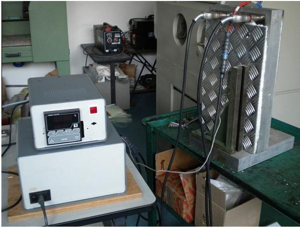
Fig. 4. Temperature control of the mold electric heater.
