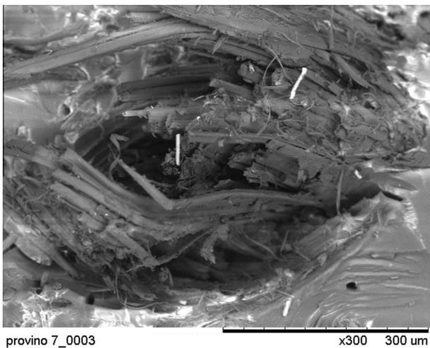
Fig. 12. Fracture surface of a tensile tested laminate.
