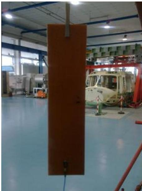
Fig. 5. Test layout for free-free vibration tests.
