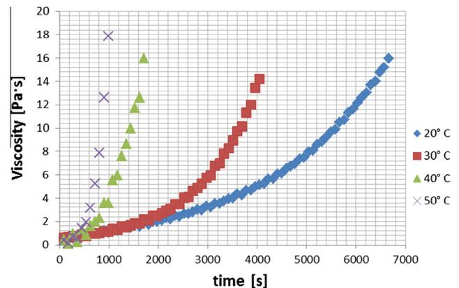
Fig. 7. Curing curves at different temperatures.
