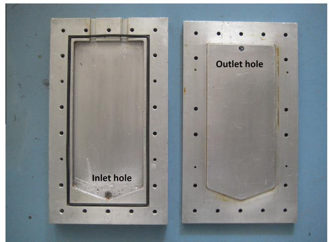
**Fig. 3.** Composite laminates production mold.
