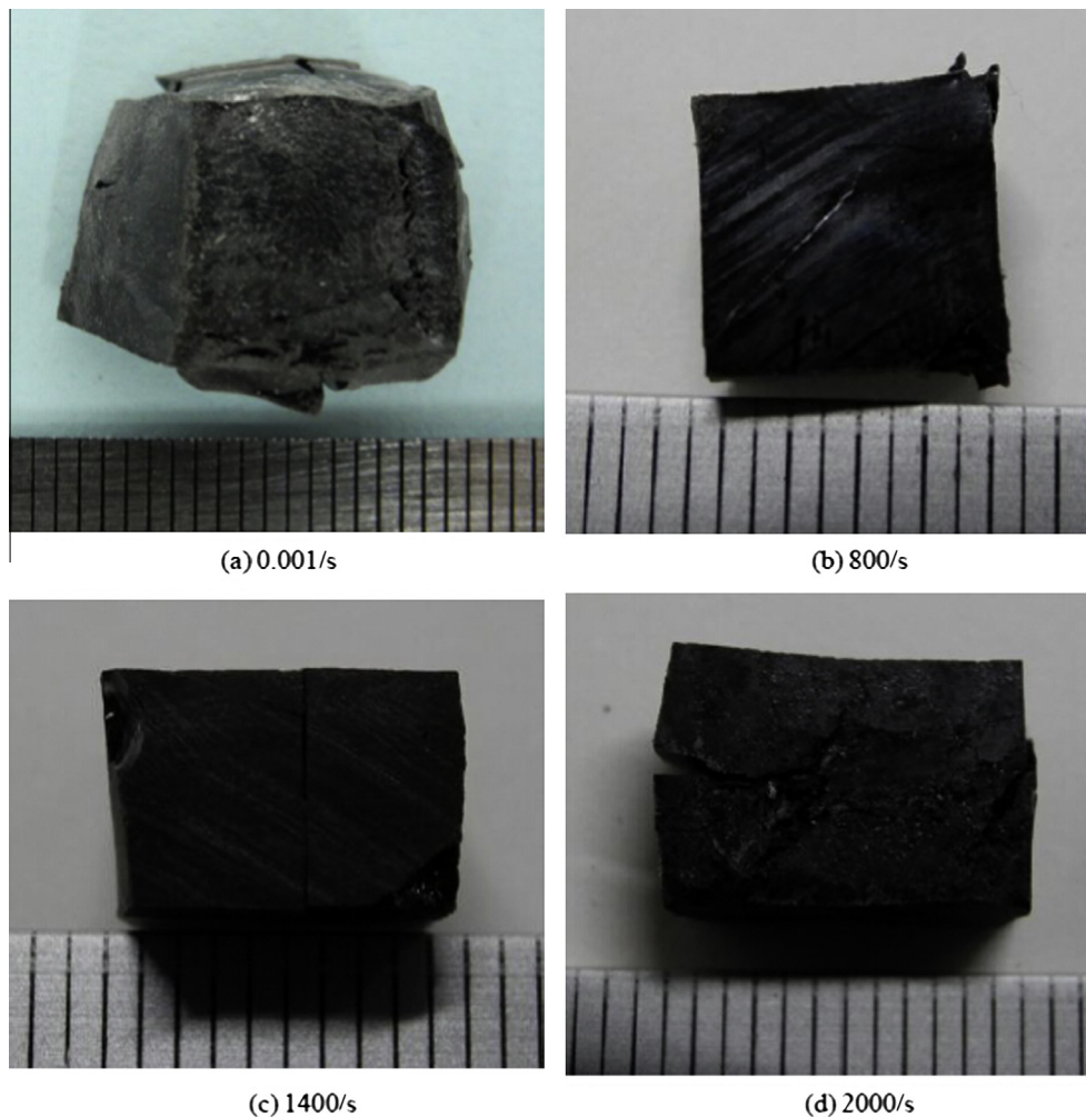
Fig. 13. Compression fractures of epoxy/CNTs (1.0 wt%) composites at various strain rates.
