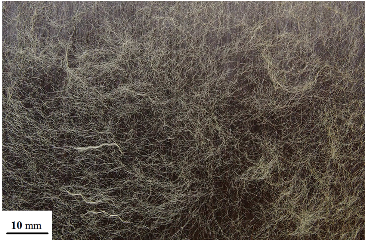
Fig. 2. Surface view of distributed short aramid-fiber tissue (fiber length: 12 mm)
