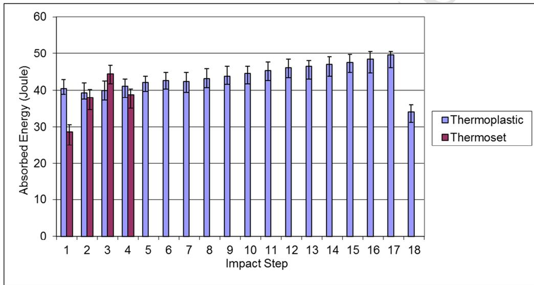
**Figure 7.** Variation of absorbed energy by impact step
