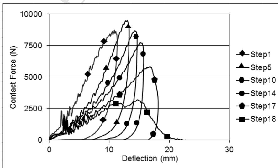
**Figure 5.** Contact force- deflection diagrams of thermoplastic composite (50 J Repeated)
