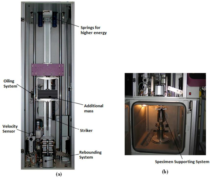
**Figure 1.** Fractovis Plus drop weight test machine
