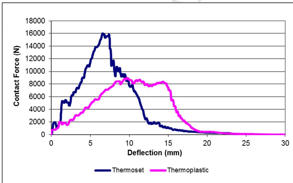
**Figure 2.** Contact force/Deflection diagram for 110 joule impact energy.
