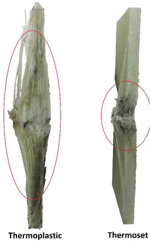
**Figure 9.** Section view of the specimens after 50 joule repeated impact tests.
