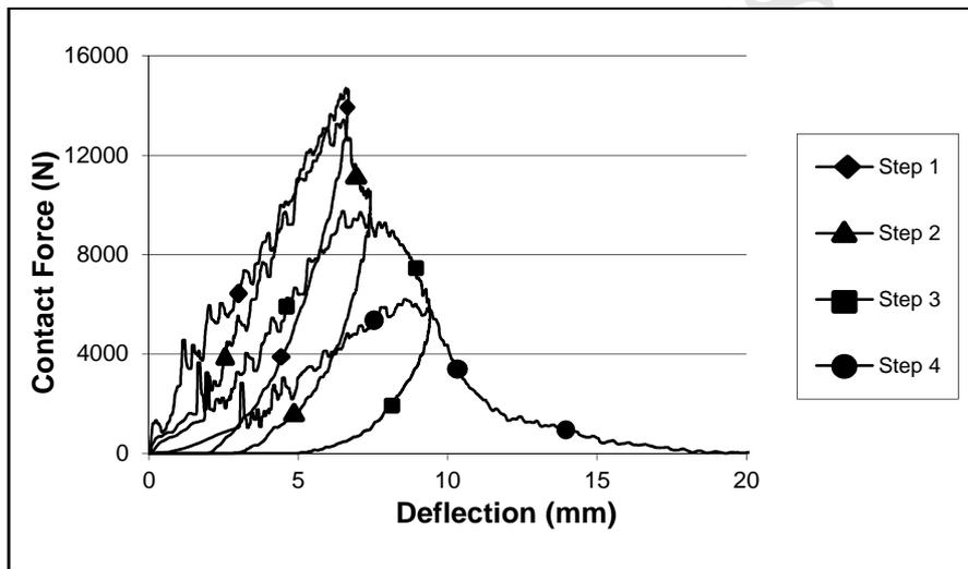
**Figure 4.** Contact force- deflection diagrams of thermoset composite (50 J Repeated)
