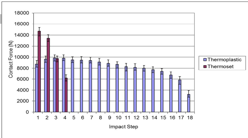
**Figure 6.** Variation of contact force by impact step
