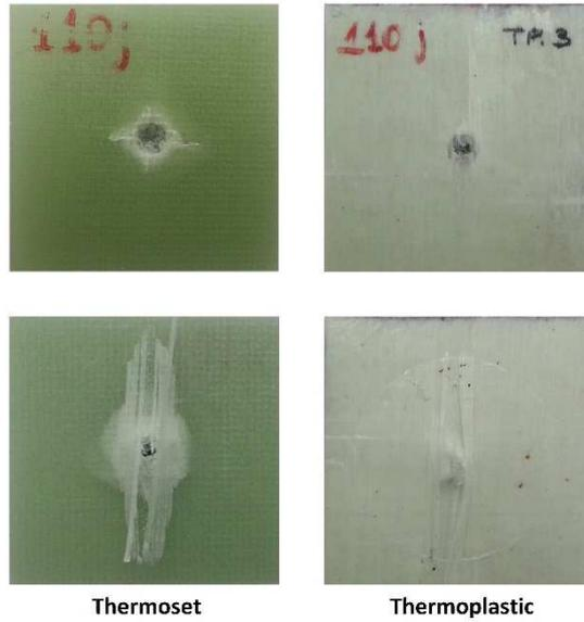
**Figure 3.** Deformation of the specimens after 110 J impact tests.
