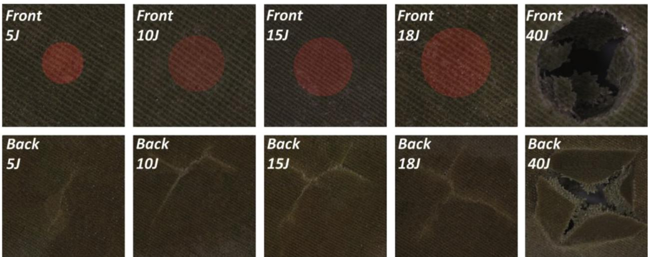
Fig. 5. Close-up views of damage progression on front and rear faces of hemp/epoxy composites impacted in the range 5 J–40 J.
