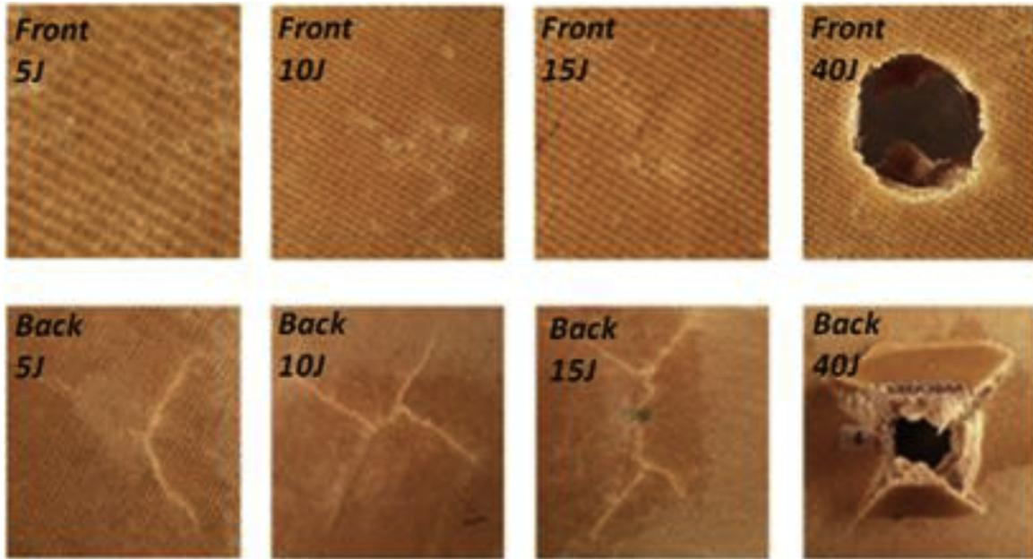
Fig. 4. Close-up views of damage progression on front and rear faces of hemp/bioepoxy composites impacted in the range 5 J–40 J.
