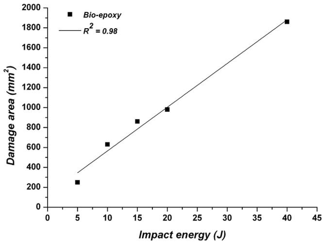
Fig. 7. Projected damage area vs. impact energy.
