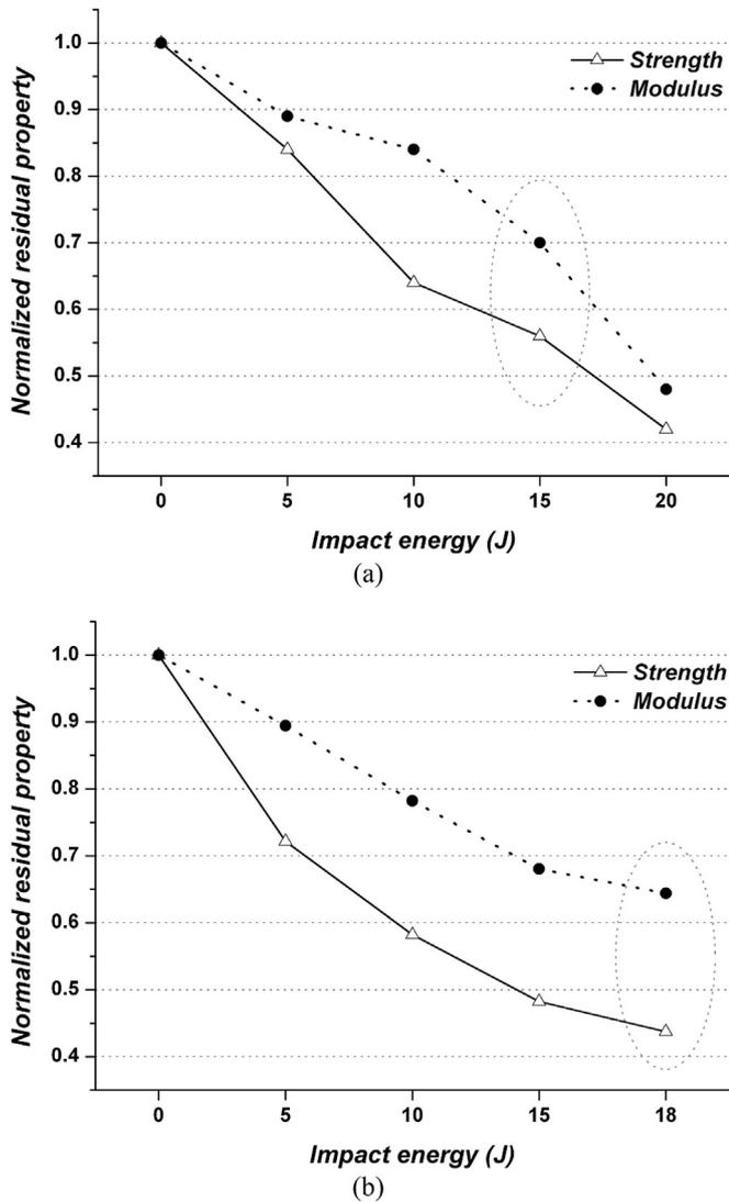
**Fig. 10.** Normalized residual flexural strength and modulus of hemp fibre reinforced composites after low velocity impact of various energies: (a) bioepoxy matrix and (b) traditional epoxy matrix.
