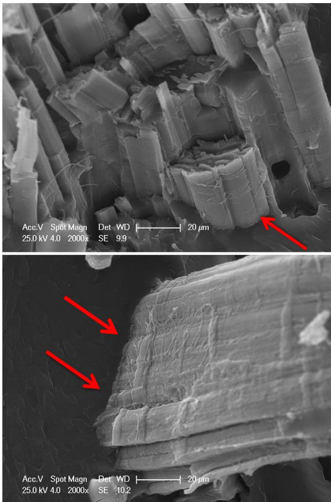
Fig. 8. SEM micrographs showing fracture surfaces of hemp/bioepoxy laminates.
