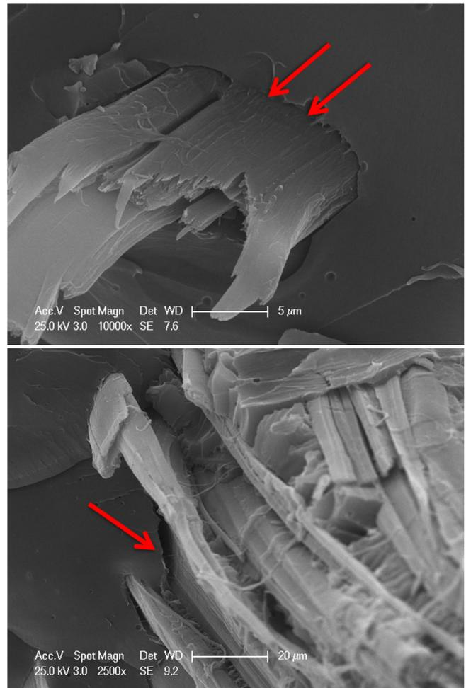
Fig. 9. SEM micrographs showing fracture surfaces of hemp/epoxy laminates.
