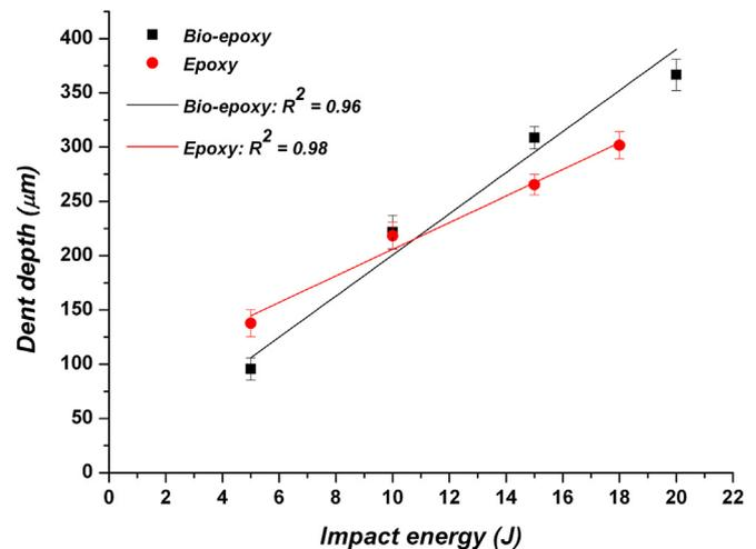
Fig. 3. Dent depth vs. impact energy.
