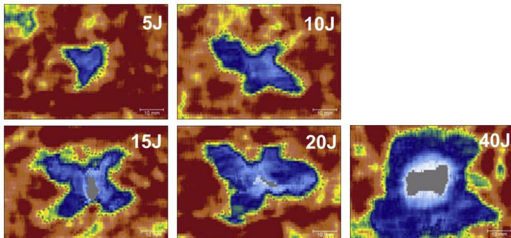
Fig. 6. Ultrasonic C-scan images of composites based on bioepoxy as a function of impact energy.
