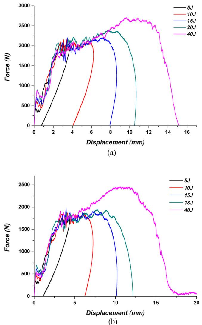
Fig. 2. Typical force vs. displacement response as a function of impact energy of composites based on (a) bio- and (b) traditional epoxy matrix.
