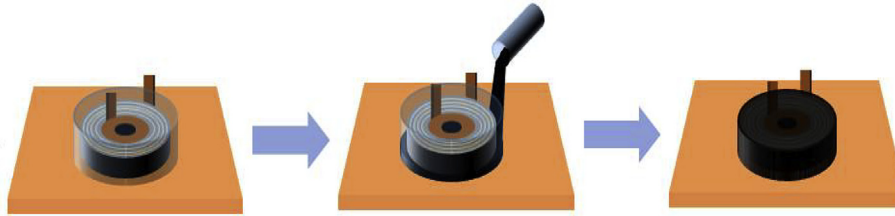
Fig. 2. A schematic drawing of the impregnating procedure for the test coil.
