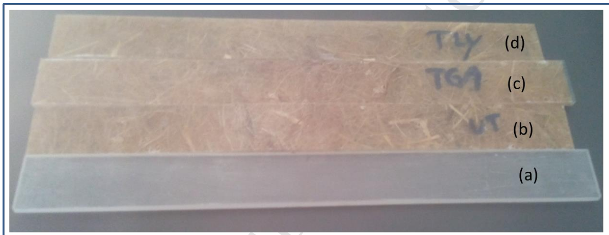
Fig. 3. Specimens used for testing; (a) Epoxy Resin, (b) Untreated Kenaf fiber, (c) Treated fiber with Glutamic acid, (d) Treated fiber with Lysine
