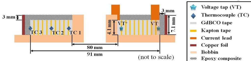
Fig. 2. Schematic cross-sectional view of the test coil impregnated with the epoxy composite.
