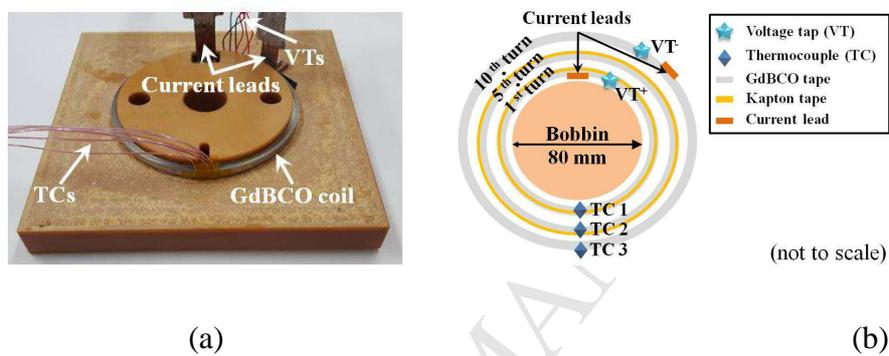
Fig. 1. Photograph of the GdBCO test coil before epoxy impregnation (a) and a schematic drawing of the instrumentation consisting of the array of E-type TCs and VT (b).
