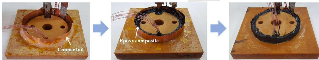
Fig. 3. Photographs of the test coil during impregnation procedure.
