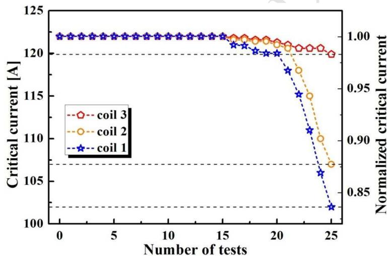
Fig. 8. Repetitive-cooling test results for coils 1, 2, and 3.
