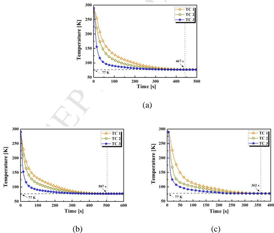
Fig. 6. Cooling test results of coil 1 (a), coil 2 (b), and coil 3 (c) obtained during cool-down from room temperature to 77 K.
