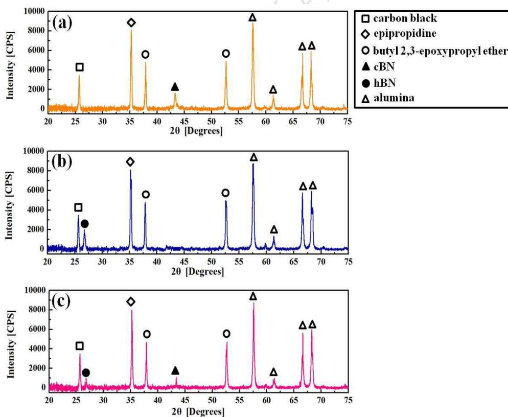
Fig. 4. XRD patterns: (a) epoxy/cBN, (b) epoxy/hBN, and (c) epoxy/cBN–hBN composites.
