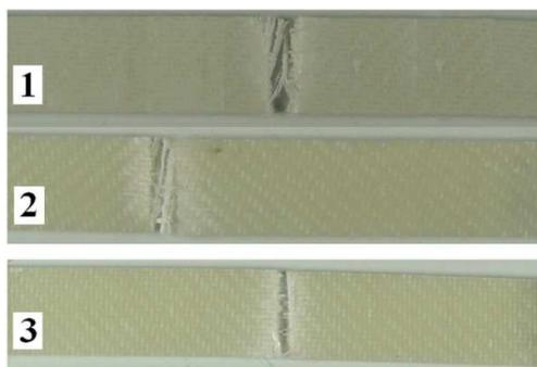
**Fig. 6.** Selected composite specimens after tensile test: 1-ASET, 2-5APP, 3-5PNA.
