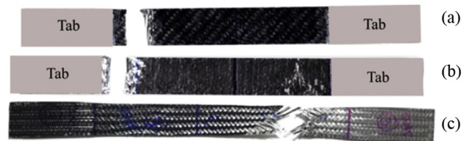
Fig. 4. Macroscopic fracture: (a) CG^C ; (b) CG^G ; (c) CG^{\pm 45^\circ} .
