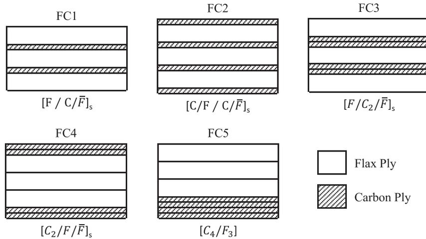
Fig. 1. Schematics indicating the stacking sequences of hybrid flax-carbon epoxy laminates.
