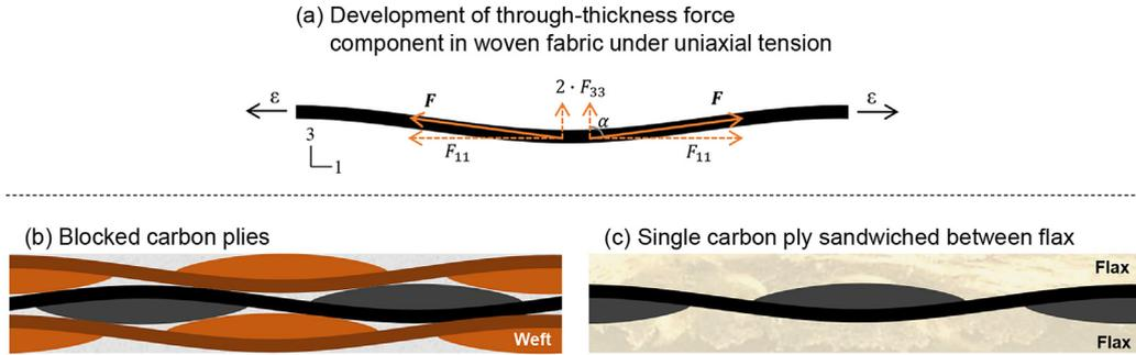
**Fig. 5.** Development of out-of-plane normal force component in woven fabric under uniaxial tension resulting in dissimilar out-of-plane deformation when carbon plies are (b) blocked and (c) interspersed between flax plies. For the same relative flax-carbon fiber volume fractions, out-of-plane deformation is more pronounced in (c) where single carbon ply is sandwiched by more compliant flax epoxy than the stiff and densely packed carbon fibers in (b).
