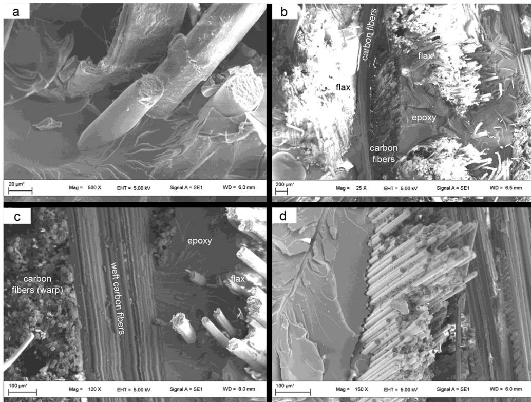
**Fig. 13.** Fracture surface morphology of composites failed under tension, illustrating (a) flax epoxy, (b) flax-carbon epoxy hybrid, magnified in (c), and (d) carbon fiber-matrix interfacial crack.
