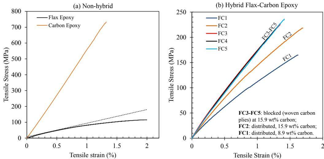
Fig. 4. Stress-strain characteristics of (a) non-hybrid flax and carbon epoxy, (b) hybrid laminates FC1-FC5 under tension.
