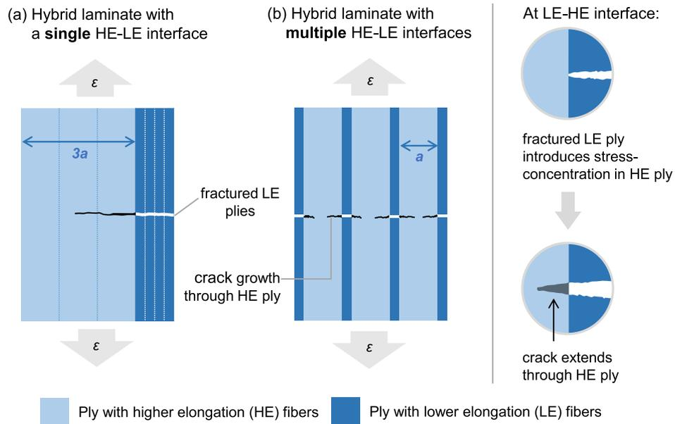
Fig. 9. Progressive failure post LE-ply rupture in hybrid laminates with (a) single, and (b) multiple LE-HE interface(s).
