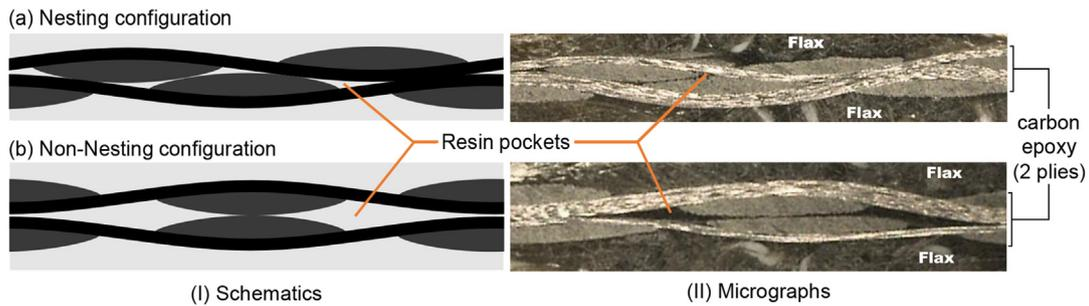
**Fig. 6.** (I) Schematics illustrating interlayer (a) nesting, and (b) non-nesting configurations in woven carbon epoxy plies. (II) Micrographs of two carbon epoxy plies sandwiched between flax in hybrid laminates.
