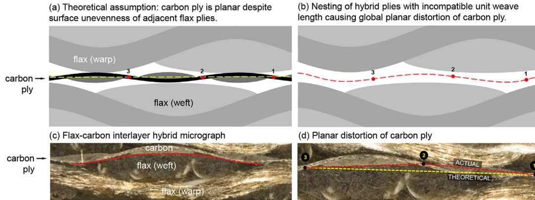
Fig. 8. Planar distortion of thin carbon plies sandwiched by flax plies due to crimp mismatch in the plain woven fabrics. 16.
