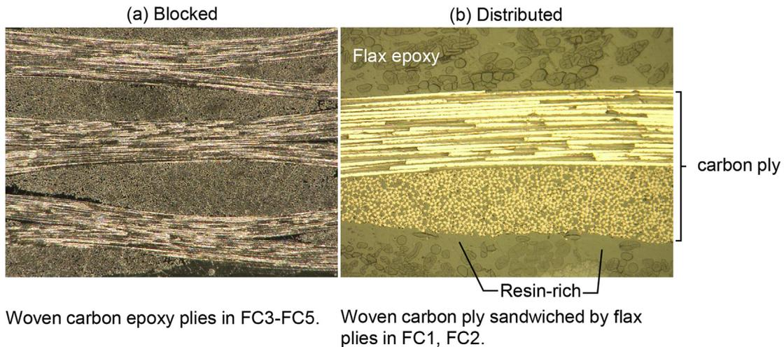
**Fig. 7.** Micrographs illustrating dissimilar out-of-plane normal boundary conditions for a woven carbon ply when (a) blocked, and when (b) distributed throughout flax-carbon interlayer hybrid laminates. Carbon ply sandwiched by densely packed stiff carbon fibers in (a), and by sporadically distributed flax fibers with relatively high resin-rich zones in (b).
