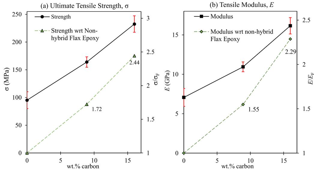
Fig. 3. Effect of carbon fiber volume fraction on tensile strength and modulus of flax-carbon hybrid composite.  $\sigma_F$  and  $E_F$  are strength and modulus of non-hybrid flax epoxy.
