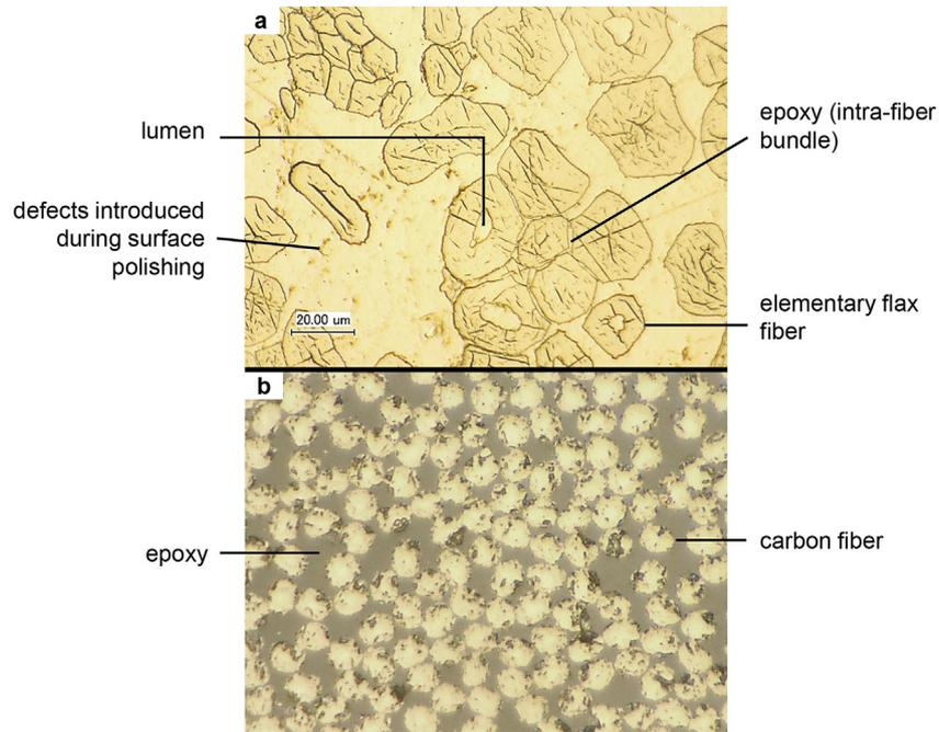
Fig. 11. Optical microscopy of the cross-sections of (a) flax epoxy, (b) carbon epoxy.
