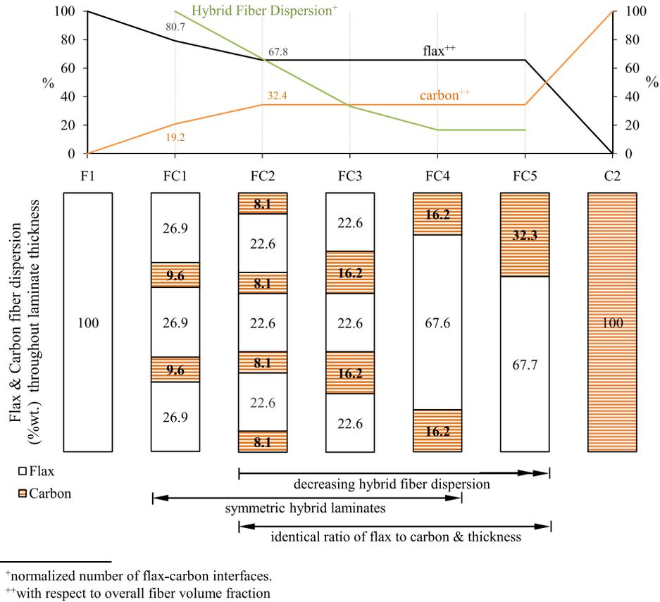
Fig. 2. Dispersion of flax and carbon fibers throughout laminate thickness in interlayer hybrids.
