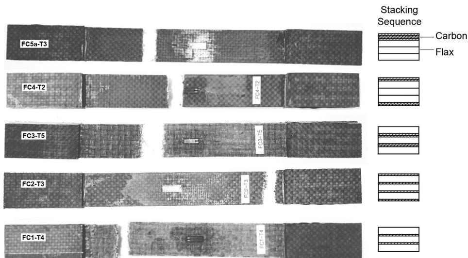
Fig. 10. Failed interlayer hybrid flax-carbon epoxy samples under uniaxial tension.
