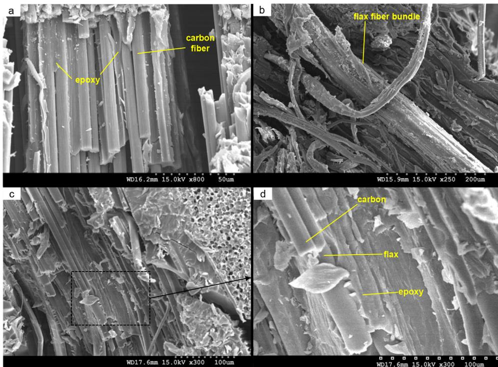
Fig. 12. SEM micrographs of (a) fibers in carbon-rich and in (b) flax-rich zones, (c) flax-carbon interlaminar hybrid zone, magnified in (d) illustrating the physical proximity of dissimilar fiber types.
