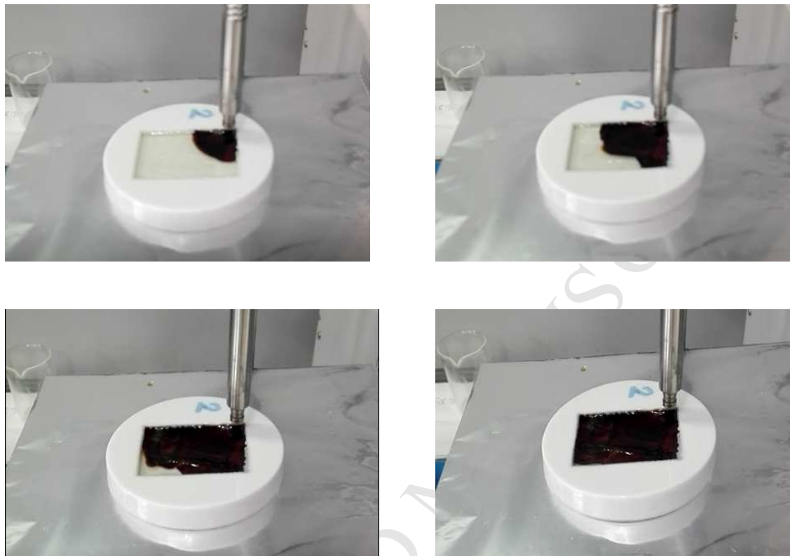
Figure 2: Pictures extracted by a movie registered during the polymerization of epoxy composites prepared with two plies of glass fibre disposed with orientation of 0^\circ and 90^\circ . Lamp turn-on for 10 seconds.
