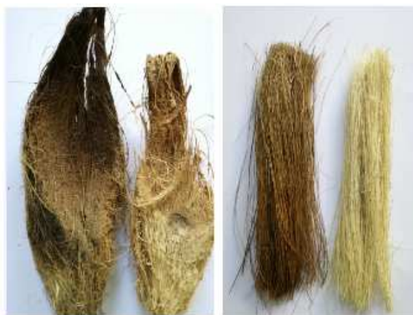
Fig. 1 Brown and white coir: fibres removed from coconut (left), fibres prepared for experimental program (right)
