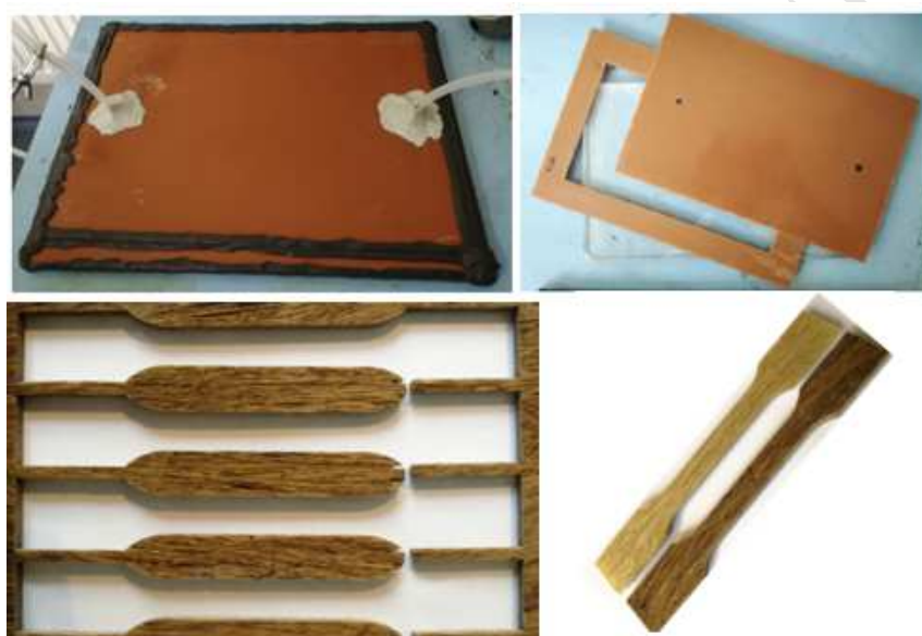
Fig. 6 Process of composite board preparation and cutting test samples by water jet
