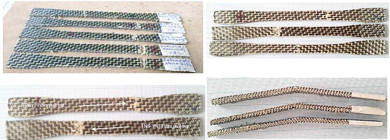
Fig.6. Failure types of composites after the mechanical tests.
