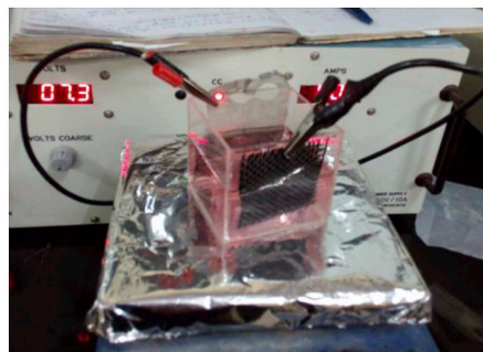
Scheme 1. Schematic representation of lab-scale electrodeposition setup.
