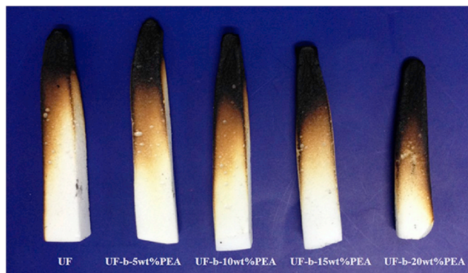
Fig. 12. Photographs of neat UF and UF-b-PEA foams after UL-94 test.
