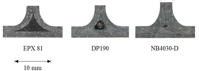
Figure 19: Close-up of deltoid areas filled with the different deltoid materials
