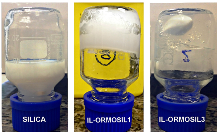
Fig. 2. Visual aspect of the IL-ORMOSILs prepared by the one-pot sol-gel route.
