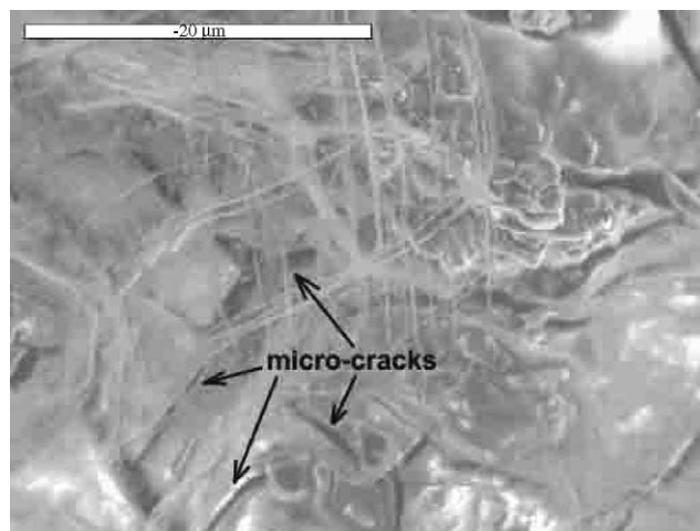
Fig. 1. Micrograph of bonding interface treated at 800 °C.
