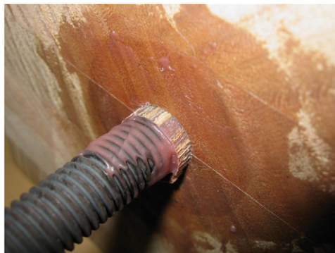
Fig. 3. Failure mode in eucalyptus specimens.
