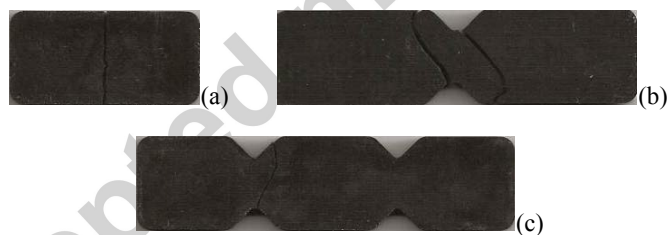
Fig. 3. Characteristic failure modes of the epoxy composite for the (a) three point-bending, (b) Iosipescu and (c) double v-notch test methods.
