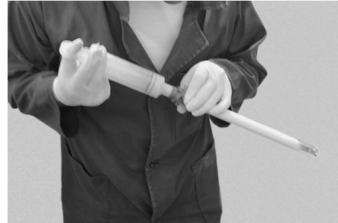
Fig. 5. Photo of the epoxy injection into the acrylic tube.
