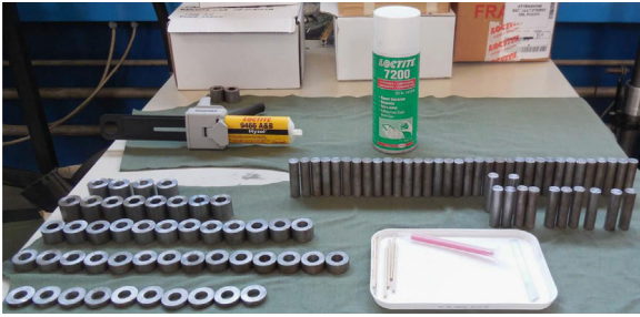
Fig. 3. Pin and collar samples with the assembly tools.
