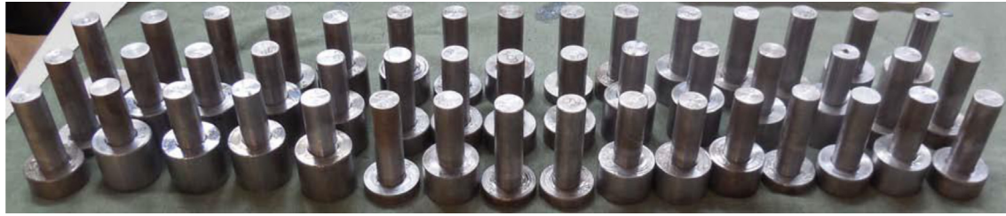
Fig. 4. Pin and collar samples assembled before the pushing-out operation.
