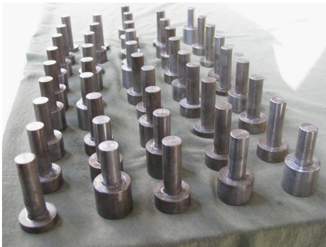
Fig. 1. An overview of the specimens, after pin-collar coupling, before the campaign at 40 °C.
