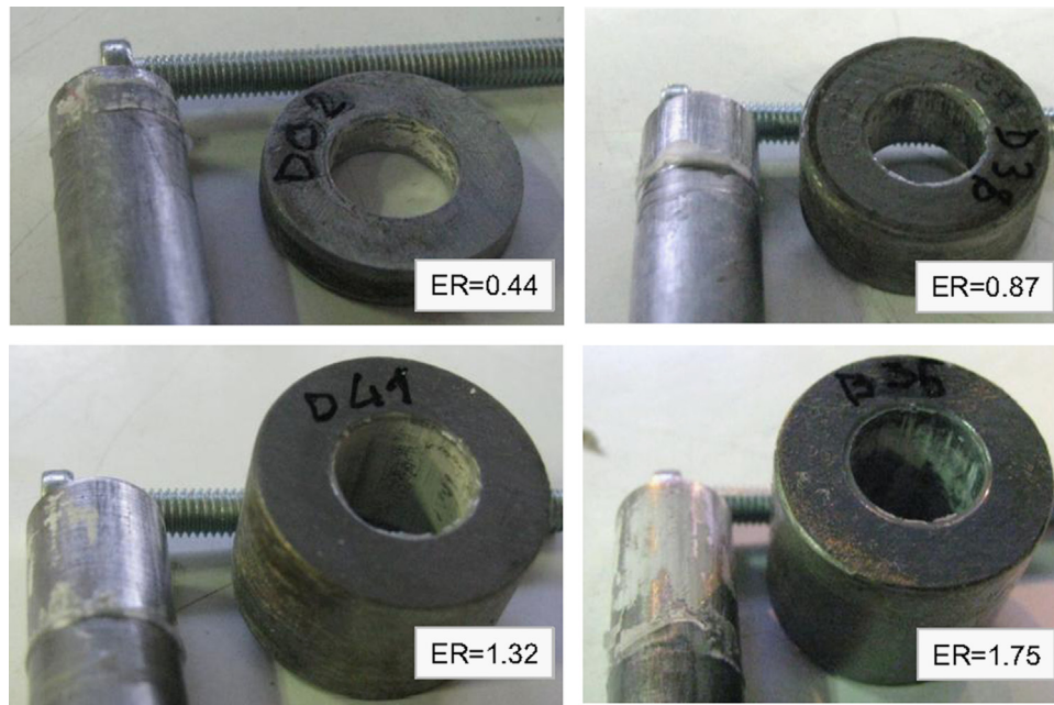
Fig. 4. Some specimens with different ERs after decoupling at the temperature of 80 °C.
