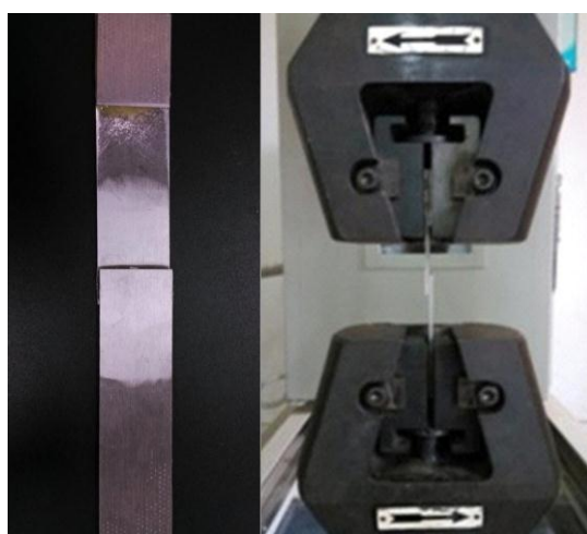
Fig. 2. The CMT-5105 universal electronic testing machine.
