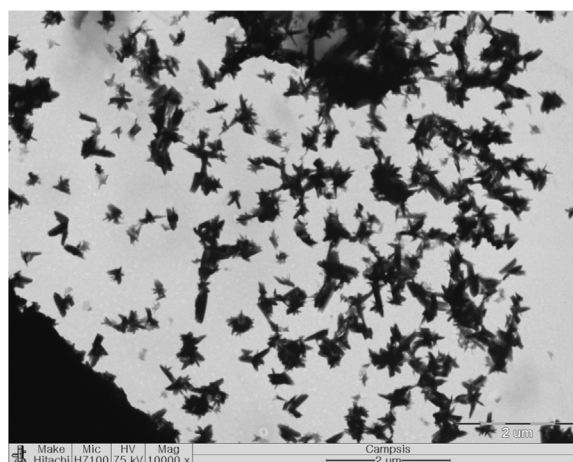
Fig. 8. Liquid UF resin of 1.0 F/U mole ratio with 5% NH 4 Cl, crystals appear to form variable size aggregates.
