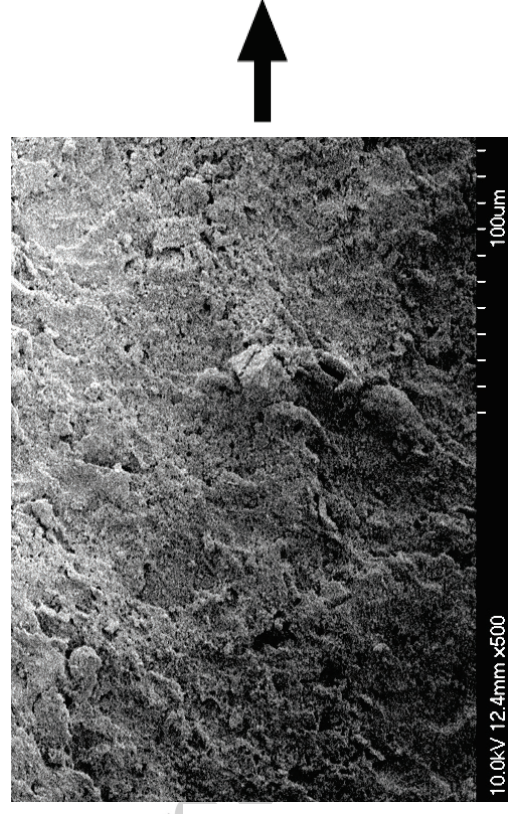
(b) Epoxy adhesive under tensile loading
