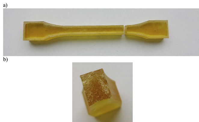
Fig. 17. Failure of epoxy adhesive composition - Specimen 7 (Epidian 5/PAC/100:70): a) Specimen 7 after destructive test, b) cohesive failure of two part of Specimen 7.
