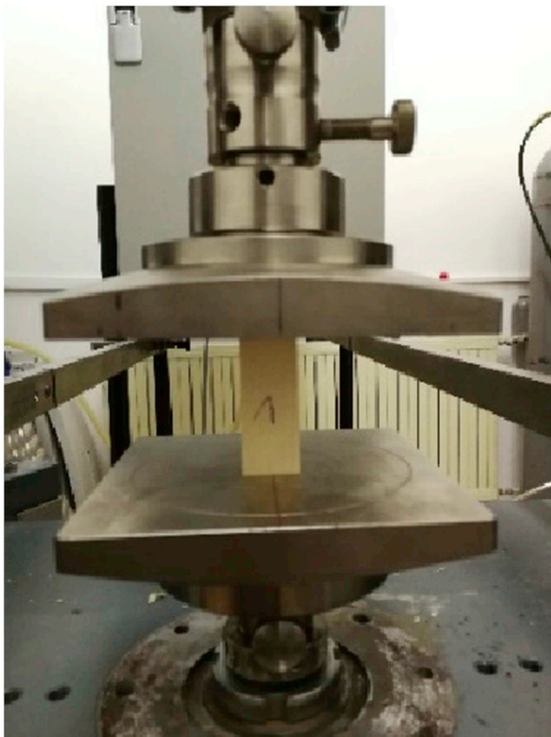
Fig. 4. Timber sample compressive test.
