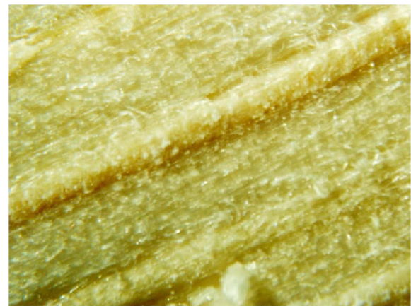
Fig. 10. The ruptured timber surface (with latewood peaks).
