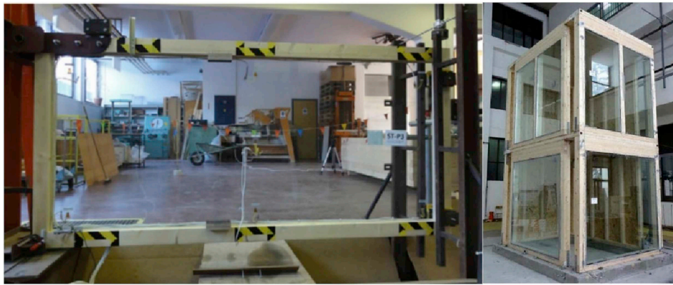
Fig. 1. Timber-glass wall panel static racking test (adopted from Ber et al. [5]) and two-story timber-glass building shaking table test (adopted from Ber et al. [7]).
