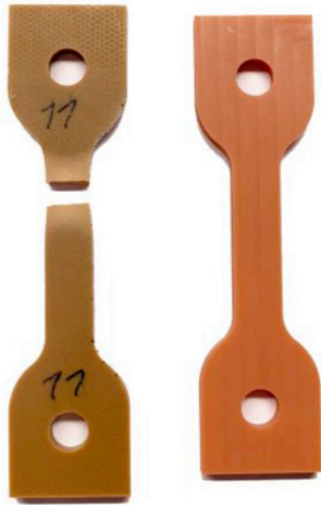
Fig. 6. Irradiated specimen after tensile test (left) and non-irradiated specimen (right).
