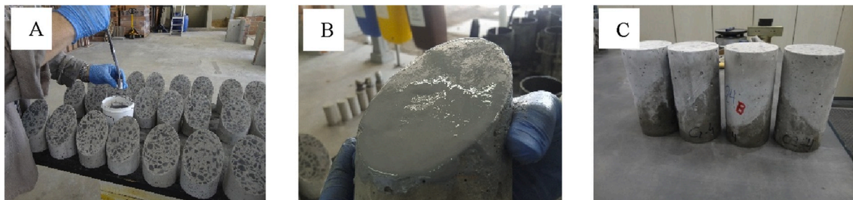
Fig. 5. Shows a) base samples cut at 45°. b) epoxy adhesive layer applied over the base. c) mixed specimens (with or without adhesive).
