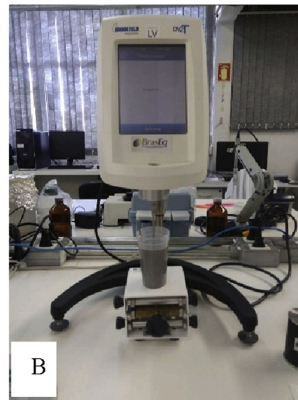
Fig. 2. Viscosity measurement of the 6 epoxy adhesives studied using a) IKA mechanical stirrer model RW20 digital b) DV2T Brookfield rotational viscometer.
