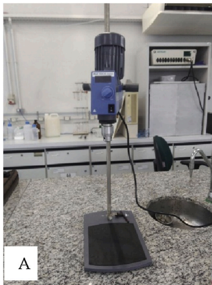
Fig. 2. Viscosity measurement of the 6 epoxy adhesives studied using a) IKA mechanical stirrer model RW20 digital b) DV2T Brookfield rotational viscometer.
