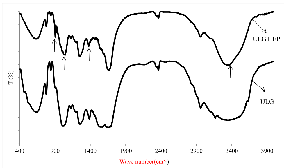
Fig. 1. FTIR analysis of ULG resin and ULG resin with epoxy.
