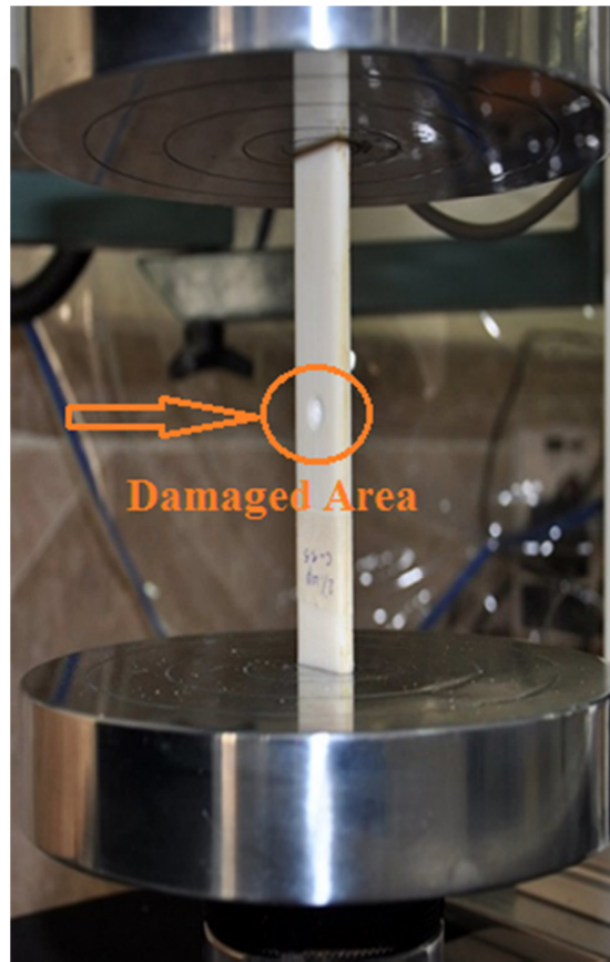
Fig 8. Damaged laminate under buckling test
