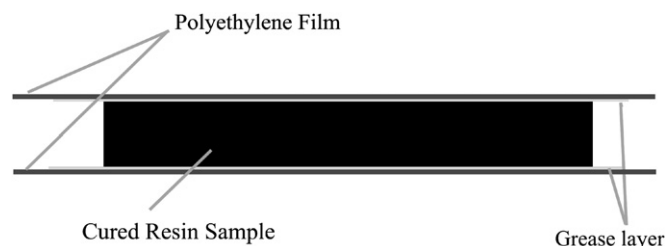
Fig. 1. Schematic of the specimen with coatings in preparation for DMTA.
