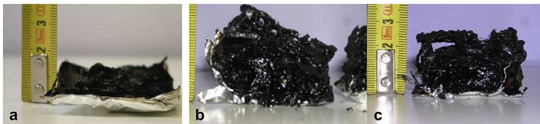
Fig. 4. Cross sections of cone calorimeter residues of POSS-epoxy hybrid systems: (a) neat epoxy matrix, (b) 3.7 inorg. wt% pre-reacted Gly-Ph POSS, (c) 3.7 inorg. wt% OctaPh POSS.
