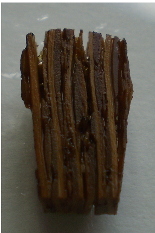
Fig. 9. Composite sample made of resin C after 240 min at 275 °C (14,937 s including heating phase).
