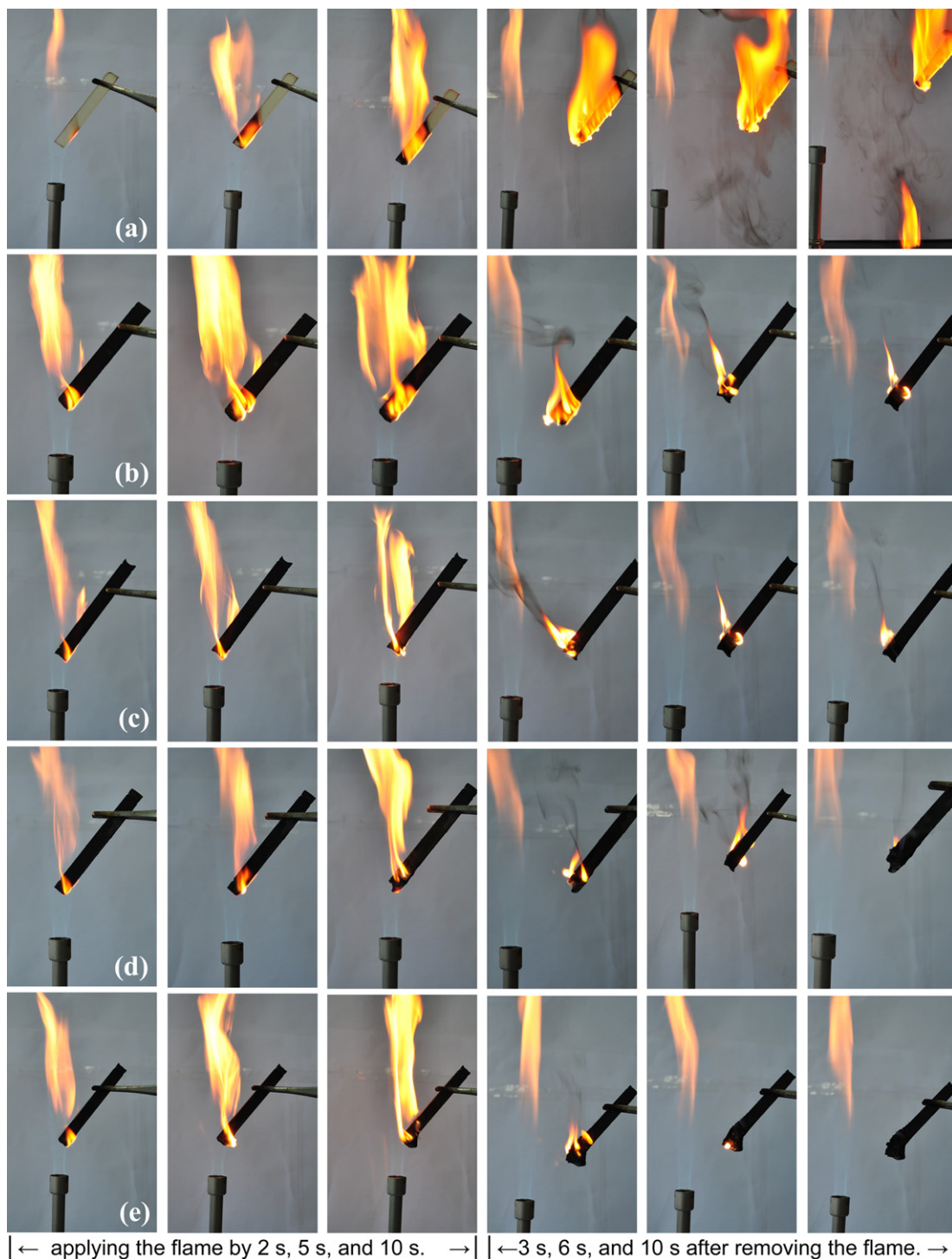
Fig. 13. Digital photographs of the combustion procedures of (a) conventional DGEBA thermostet and DGEBA/PN–EPC thermostets containing (b) 5 wt.%, (c) 10 wt.%, (d) 15 wt.%, and (e) 20 wt.% of PN–EPC under a vertical burning condition.
