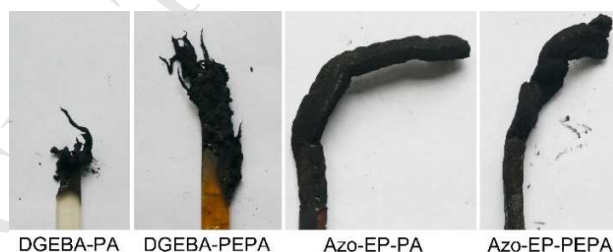
Fig. 4. Burning residues after LOI test of DGEBA-PA, DGEBA-PEPA, Azo-EP-PA and Azo-EP-PEPA
