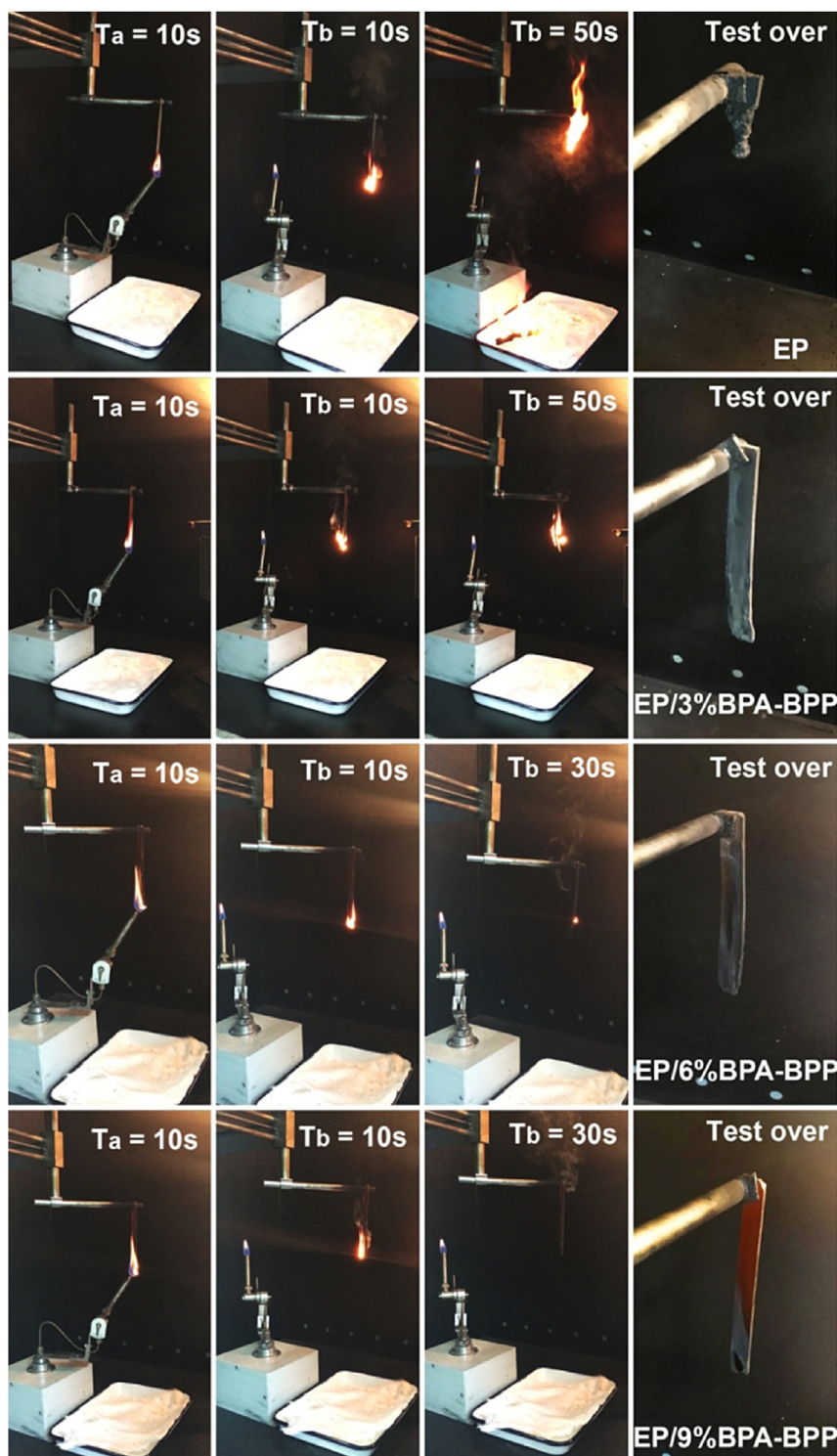
Fig. 6. Photographs of the EPs recorded during UL-94 tests. T_a , the first 10 s ignition; T_b , the time after the first ignition.
