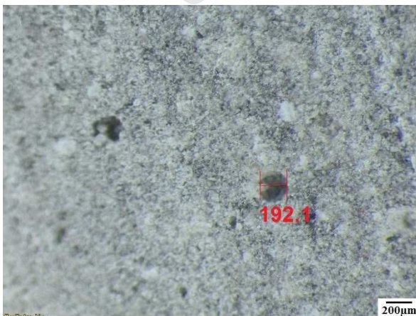
Figure 4: Porosity of F0 at elevated temperature
