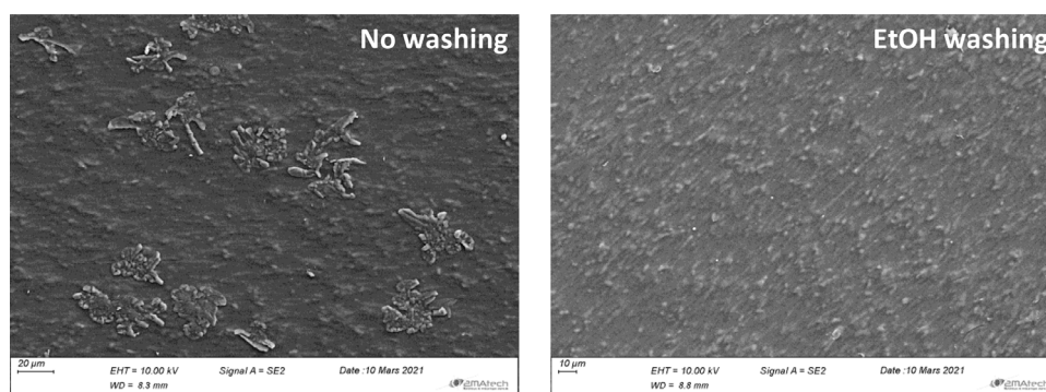
Fig. 6. SEM images ( \times 400 ) of unwashed (left) and EtOH-washed (right) PE-770-1 films.
